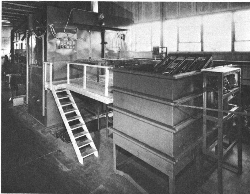
Figure 6. 76 inch diameter E. B. Blue Co. rotational casting machine
